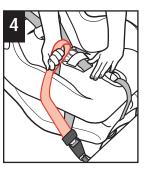
Push down firmly on the child restraint and pull up on belt to tighten. For a manual belt, refer to "Knowing your Vehicle Belt" section. Pull up on shoulder strap to remove any slack.
